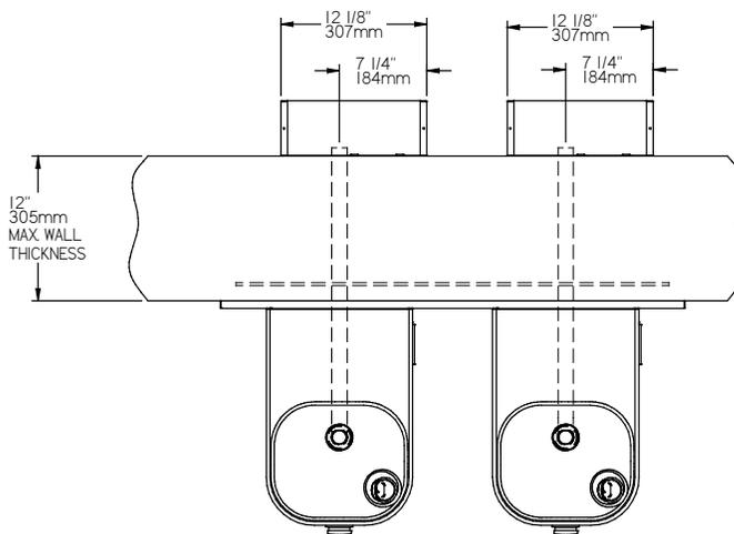
**When installing HDFFBLEBP w/FR (Carrier) with MPW200 in-wall plate mounted directly to wall studs, refer to these diagrams.**
