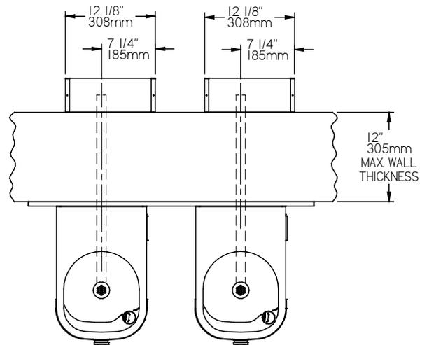
**When installing HDFFBLEBP w/FR Box which includes a surface mounting plate, refer to these diagrams.**
